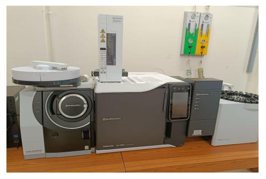
Thermal Desorption Gas Chromatography Mass Spectroscopy (TD-GCMS)
